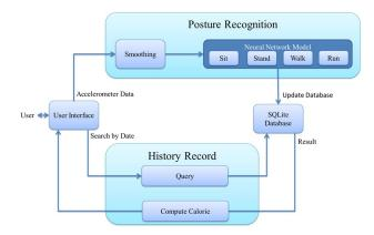
Figure 3. System architecture of the posture recognition app
